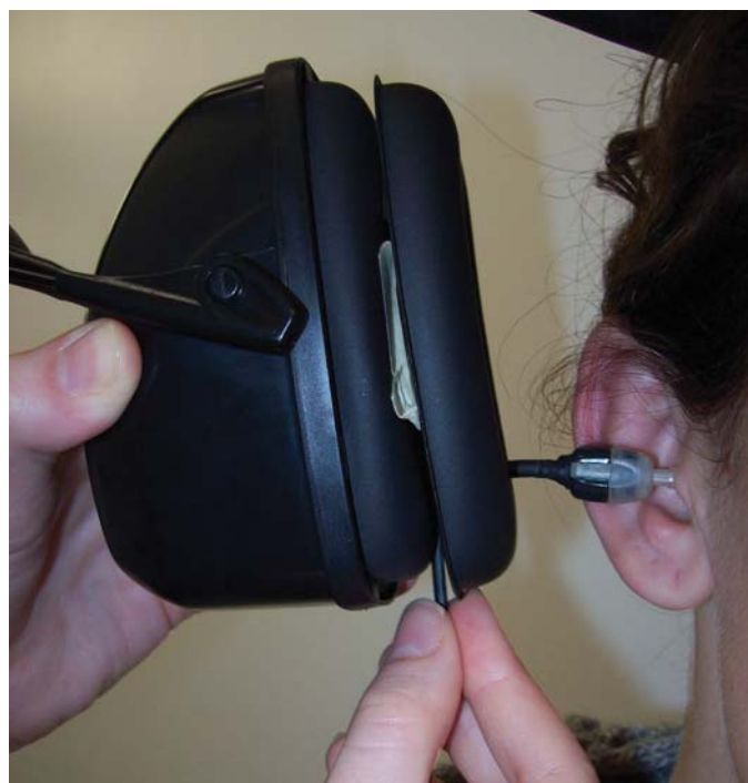
Figure 3. The DPOAE probe was inserted into the ear canal and the cord gently pulled to reduce slack and allow the probe to fit securely and comfortably in the ear canal.
