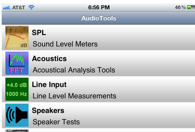
Figure 1. AudioTools App selected on iPhone. Note: To store and share your measurements, take a screen shot with your iPhone. To do this, hold the “home” button, and press the on/off button on the top. The phone will make a camera shutter sound; the resulting “photo” is now on photo roll.
