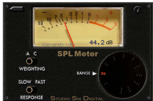
Figure 2. iPhone with Analog Sound Level Meter App running.
